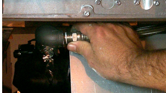
Figure 1 The oil filter carriage must be disconnected from the filter pump to be completely removed from the fryer cabinet.
