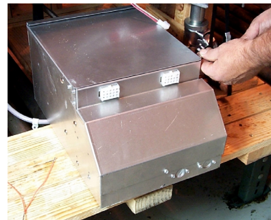
Figure 5: Remove top to gain access to connector blocks.
